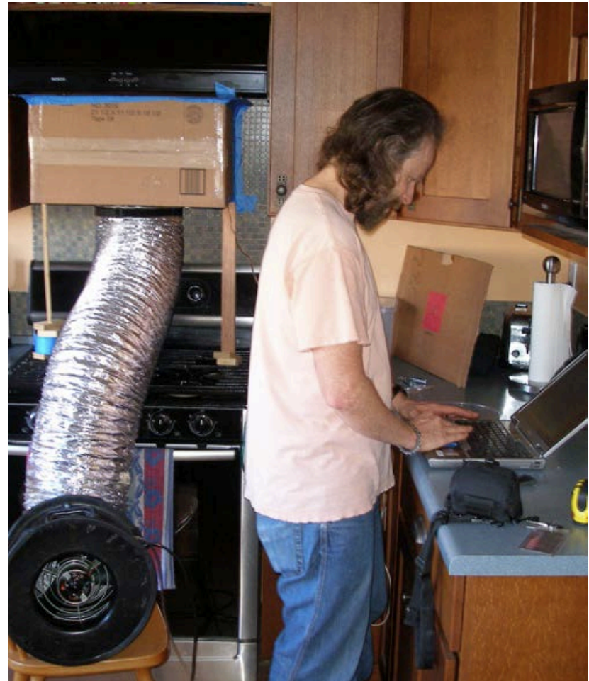
Measuring air flows with active flow hood
