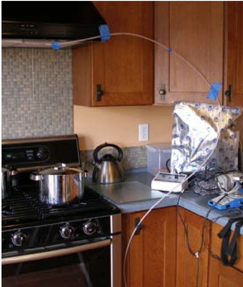
Sampling CO 2 from gas burners
