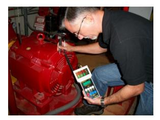
Figure 3: Vibration analysis tool indicator
