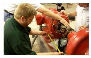
Figure 4: Laser alignment of a pump
